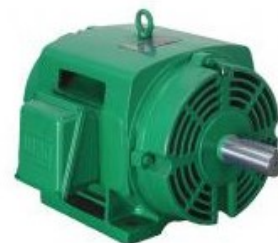
Weg 100 HP General Purpose Motor, 3-Phase, 3550 Nameplate RPM, Voltage 208-230/460, Frame 365TS - 10036OT3E365TS
