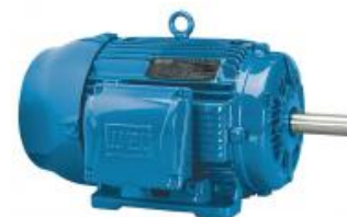
Weg 100 HP General Purpose Motor, 3-Phase, 3555 Nameplate RPM, Voltage 208-230/460, Frame 404/5TS - 10036ET3E405TS-W22
