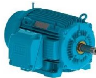
Weg 150 HP IEEE 841 Motor, 3-Phase, 3600 Nameplate RPM, Voltage 460, Frame 444/5TS - 15036ST3QIE445TS-W22
