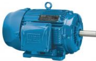
Weg 200 HP General Purpose Motor, 3-Phase, 1780 Nameplate RPM, Voltage 460, Frame 445/7T - 20018ET3G447T-W22
