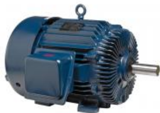
Marathon 200 HP General Purpose Motor, 3-Phase, 890 Nameplate RPM, Voltage 460, Frame 447/9T - 449TTF58110
