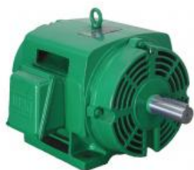
Weg 200 HP General Purpose Motor, 3-Phase, 1780 Nameplate RPM, Voltage 460, Frame 445T - 20018OT3G445T
